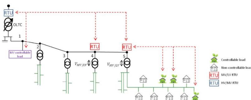
The objective of this method is to prepare flexibility provision and to plan the best economic activation of MV and LV flexibility offers to solve the cases of MV constraints deviations caused by the increased penetration of Distributed Energy Resources (DER), while ensuring that LV
